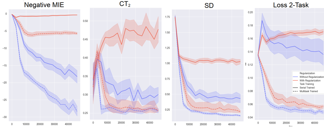
Figure 3: Network statistics (MIE, CT_2 , SD, objective loss) over the time course of training in multiclassifier networks. Units of x -axis are number of training samples. Objective loss is measured on held-out test data with samples of arity 2.
